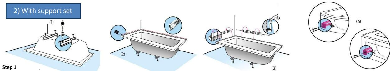
Screw the two support rods to the bottom of the bathtub and place the plastic height adjustment feet in the openings (diagram 1).
