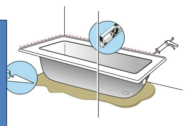
At the point where the tiles meet the bathtub, seal with <u>OTTOCHEMIE OTTOSEAL S100</u> anti-mould silicone sealant (available in various colors) using <u>OTTOCHEMIE OTTOFIMER X-PR 1216 250ml</u> primer. <u>OTTOCHEMIE OTTO-FUGENBOY Y-ZUB</u> grouting trowels and <u>OTTOCHEMIE OTTO SMOOTHING X-GL</u> liquid abrasive for easier and cleaner silicone application (see installation system).
